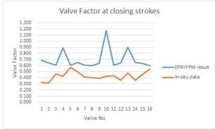
Figure 3. Valve factor at closing strokes
