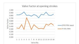
Figure 2. Valve factor at opening strokes
