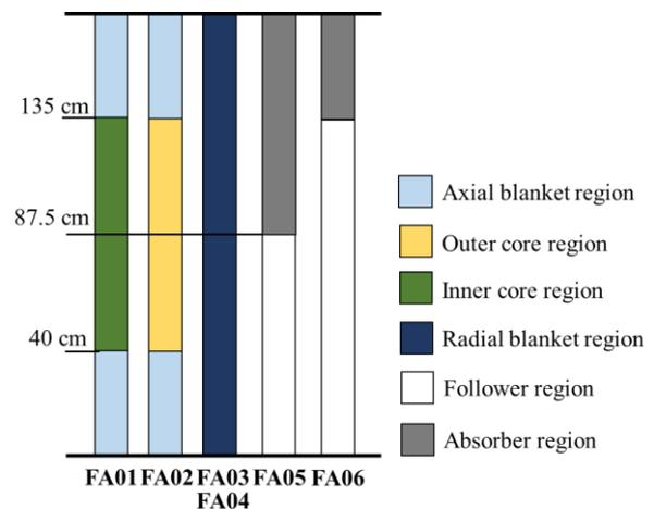
Figure 2 Axial composition of SNR
