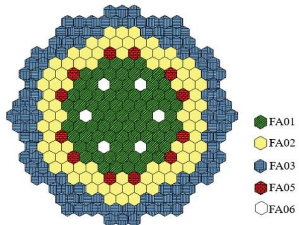
Figure 1 Loading pattern of SNR
