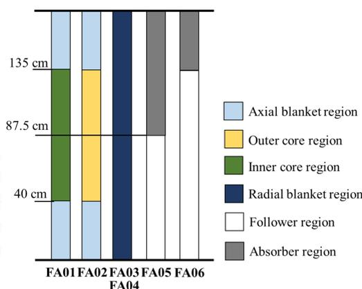
Fig. Axial composition of SNR
