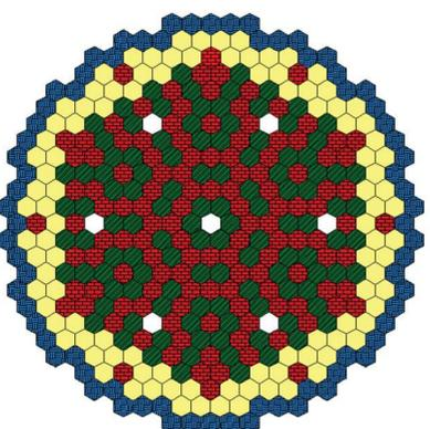
Fig. Radial layout of VVER-440
