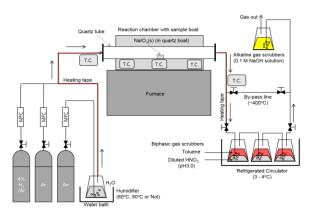
Fig. 1. Schematic diagram of thermal decomposition system
