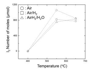
Fig. 2. Amounts of  $I_2$  formed from decomposition of NaIO<sub>3</sub> at different temperature and gas conditions
