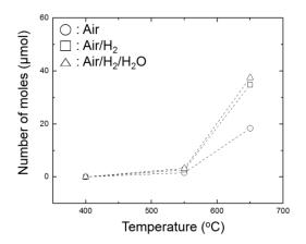
Fig. 3. Amounts of I<sup>-</sup> formed from decomposition of NaIO<sub>3</sub> at different temperature and gas conditions
