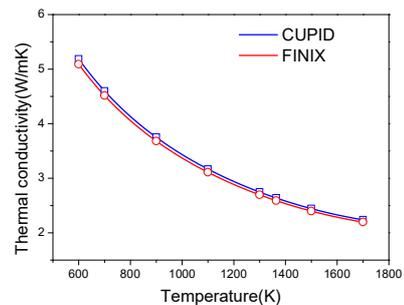
Fig. 9. Thermal conductivity distribution in CUPID and FINIX
