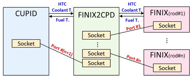
Fig. 3. Coupled scheme of CUPID-FINIX coupled code
