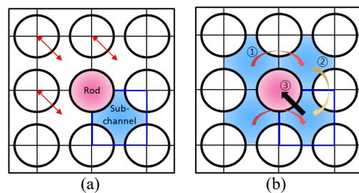
Fig. 1. CUPIDRV (a) subchannel centered geometry and rod-subchannel connectivity (b) collecting and averaging the subchannel information
