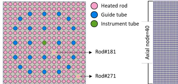
Fig. 4. VERA benchmark single assembly geometry
