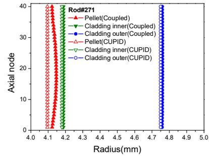
Fig. 7. Radius of pellet and cladding in CUPID standalone and CUPID-FINIX
