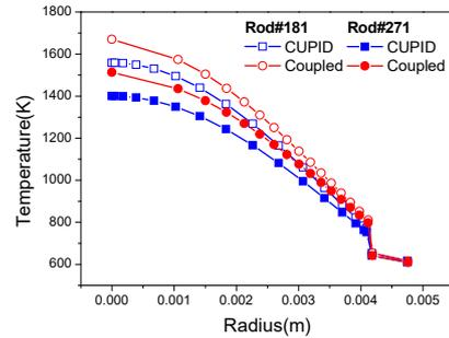
Fig. 8. Radial temperature distribution at rod 181 and 271
