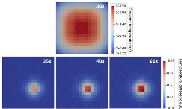
Fig. 11. Exit temperature at 30 seconds (1<sup>st</sup> steady-state) and differences (at 35, 40 and 60 seconds) from temperature at 30 seconds
