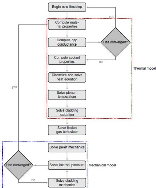
Fig. 2. Iteration scheme of FINIX code [12]
