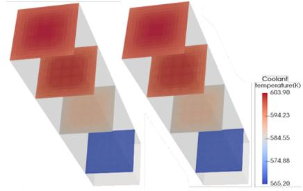
Fig. 6. Coolant temperature distribution CUPID standalone (left), CUPID-FINIX (right)
