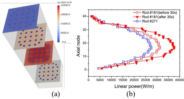
Fig. 5. Distribution of (a) volumetric heat of VERA single assembly (b) linear power at rod 181 and 271
