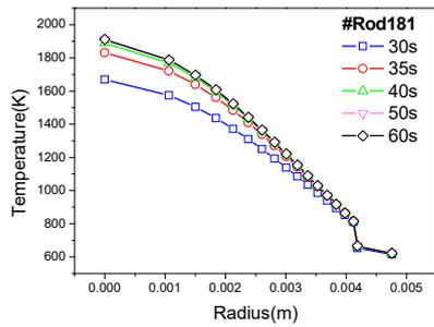
Fig. 10. Increasing radial temperature distribution over time
