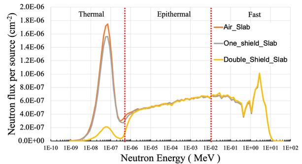
Figure 3. The neutron energy spectrum for each TLD positions calculated by MCNP6.
