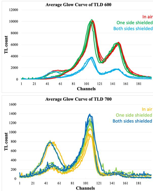
Figure 4. The averaged glow curves of TLD-600 and TLD-700 at three positions.
