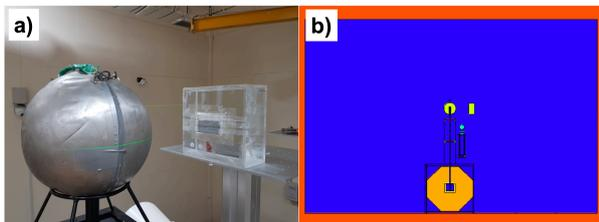
Figure 2. The TLD irradiation setup (a), The modeled geometry of irradiation room by MCNP6.
