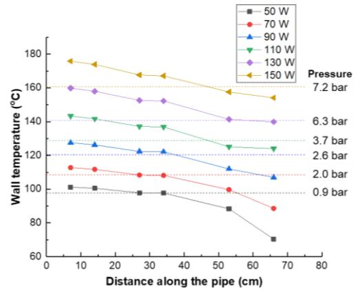
Fig. 7. Wall temperature distribution along the heat pipe for each power step.
