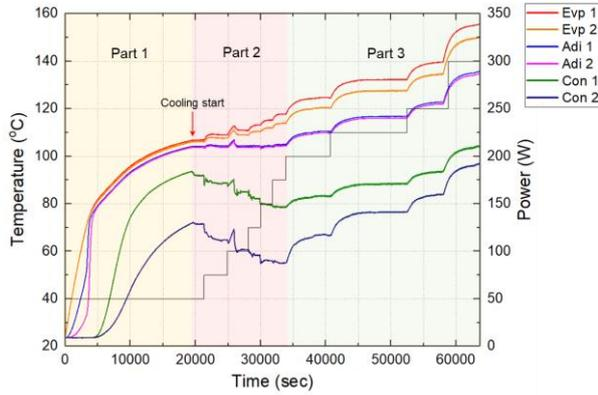
Fig. 5. Wall temperature histories of heat pipe according to heat loads.
