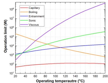
Fig. 3. Operation limits of heat pipe.
