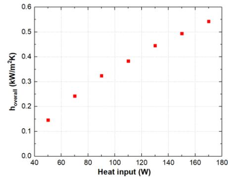
Fig. 8. Overall heat transfer coefficient of heat pipe.
