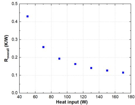
Fig. 8. Overall thermal resistance of heat pipe.
