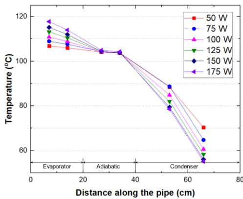
Fig. 6. Wall temperature distribution along the heat pipe for each power step.
