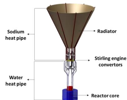
Fig. 2. Concept of heat pipe cooled space reactor. (Kilopower)
