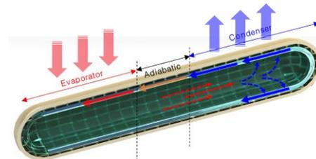
Fig. 1. Structure and working principle of heat pipe.
