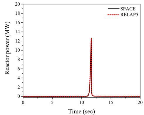
Fig. 3. Fast insertion: Reactor power
