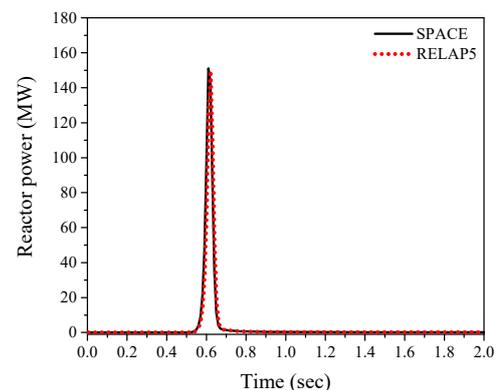
Fig. 4. Ramp insertion: Reactor power
