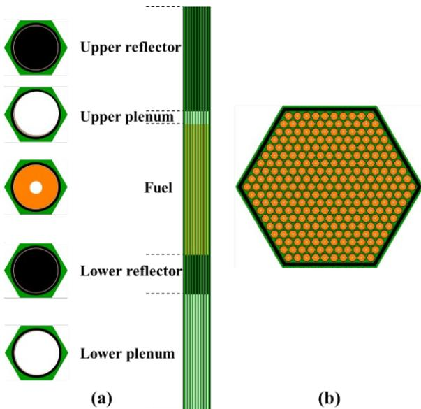
Fig. 2. Description of the fuel sub-assembly: (a) axial zones layout and (b) radial layout.
