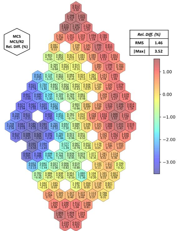
Fig. 5. Assembly power distribution at ARI state, MCS/R2 vs. MCS.
