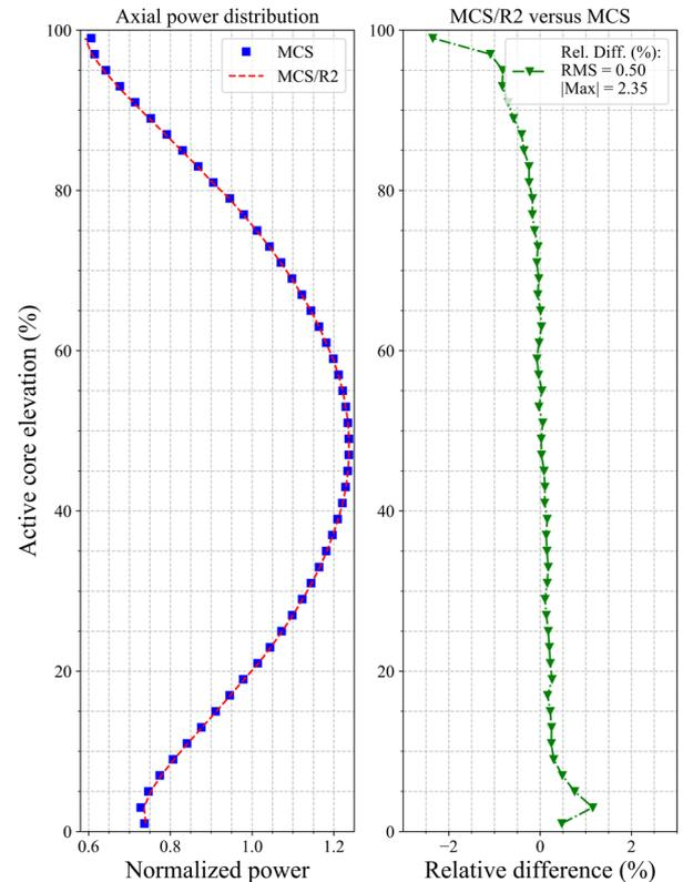
Fig. 6. Axial power distribution, MCS/R2 vs. MCS.
