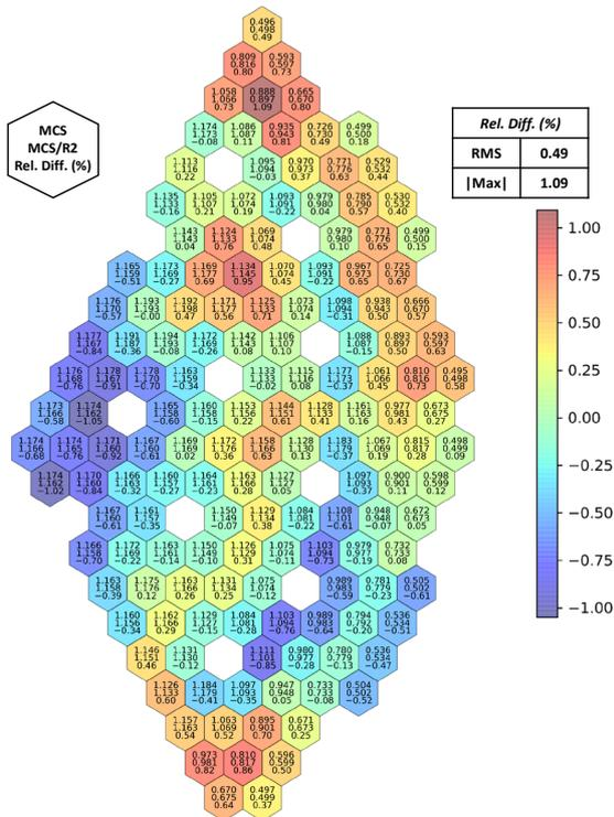
Fig. 4. Assembly power distribution at ARO state, MCS/R2 vs. MCS.
