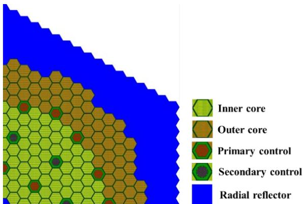
Fig. 1. Radial quarter core layout of MOX-3600.
