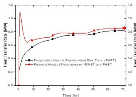
Fig. 4 Heat transfer rate
