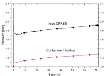
Fig. 2 Pressure inside CPRSS and containment building
