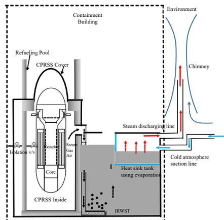
Fig. 1 Schematic of heat sink tank inside IRWST
