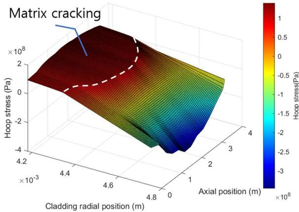
Fig. 4. Stress distribution of full  $SiC_f/SiC$  cladding in shutdown situation considering pseudo-ductility
