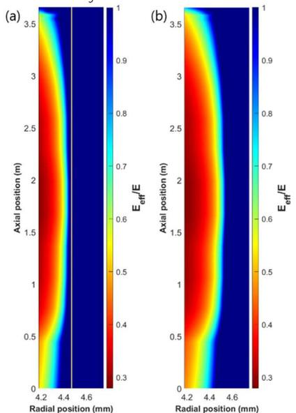
Fig. 7. Young's modulus decrease in (a) duplex and (b) full SiC<sub>f</sub>/SiC composite cladding at the end of the accident
