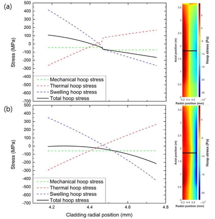
Fig. 5. Stress distribution of (a) duplex cladding (b) full  $SiC_f/SiC$  cladding in EOL
