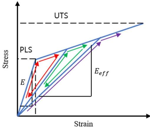
Fig. 3. Pseudo-ductile stress-strain curve
