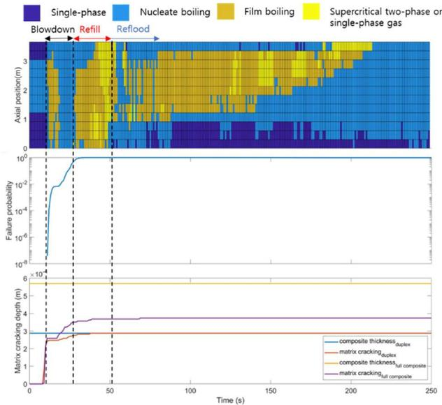
Fig. 6. (a) boiling mode, (b) failure probability of mSiC in duplex structure, and (c) matrix cracking depth depending on the elapsed time of the accident.
