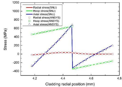
Fig. 2. Comparison of the developed model with finite element analysis solution by ANSYS: cladding thickness = 0.57 mm (CVD SiC : SiC<sub>f</sub>/SiC = 5:5),  $q' = 18$  kW/m,  $T_o = 340$  °C,  $T_{ref} = 22$  °C,  $P_i = 20$  MPa,  $P_o = 1$  MPa.
