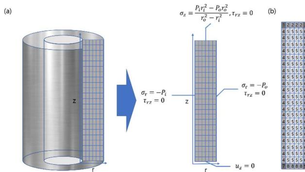
Fig. 1. (a) Boundary conditions of the axisymmetric cladding model, (b) mesh division for differentiation
