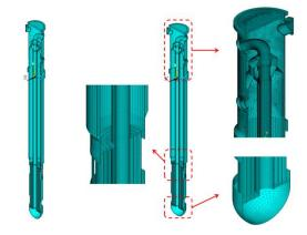
Fig. 2. Finite element model for DHX of TRU burner reactor
