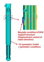
Fig. 4. Boundary condition for DHX of TRU burner reactor
