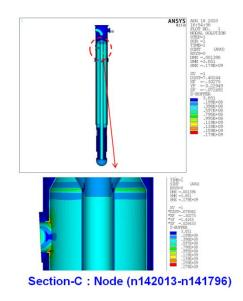
Fig. 7. Stress analysis result for Pressure
