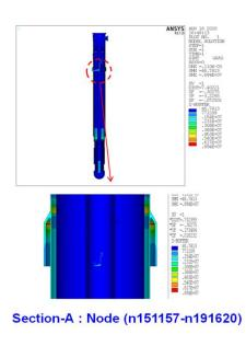
Fig. 5. Stress analysis result for dead weight
