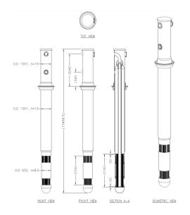
Fig. 1. Conceptual drawing for DHX of TRU burner reactor
