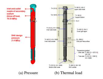
Fig. 3. Applied load for DHX of TRU burner reactor
