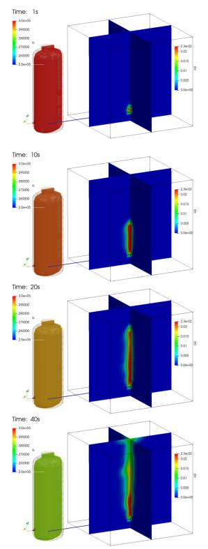
Fig. 2. MELCOR-ContainmentFoam coupled analysis, pressure field in SPARC and hydrogen distribution in the compartment along time.
