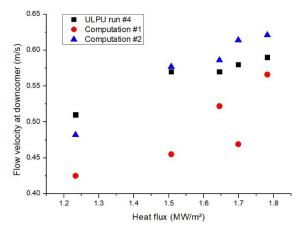
Fig. 5. Comparison of the liquid velocity applying UDF in the downcomer.
