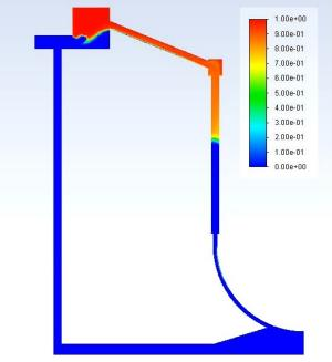
Fig. 6. Liquid volume fraction in the cooling loop; Heat flux=1.233  $MW/m^2$
