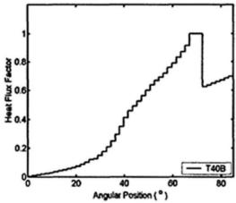
Fig. 4. Angular dimensionless heat flux profile. 7)
