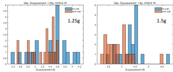
Fig. 8. Effect of moat wall (isolator model: HHHDR, CHS=3.1ft)
