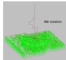
Fig. 4. ANT model with 486 isolators
