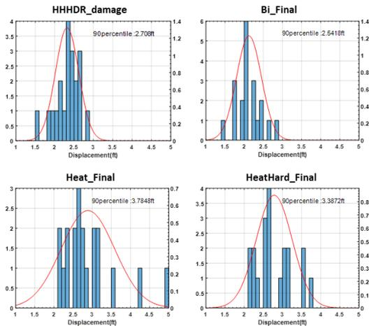
Fig. 7. Maximum displacement distribution (PGA=1.0g)
