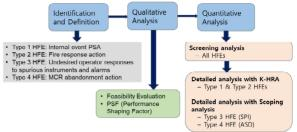
Fig 1. Overview of Fire HRA Guideline developed by KAERI
