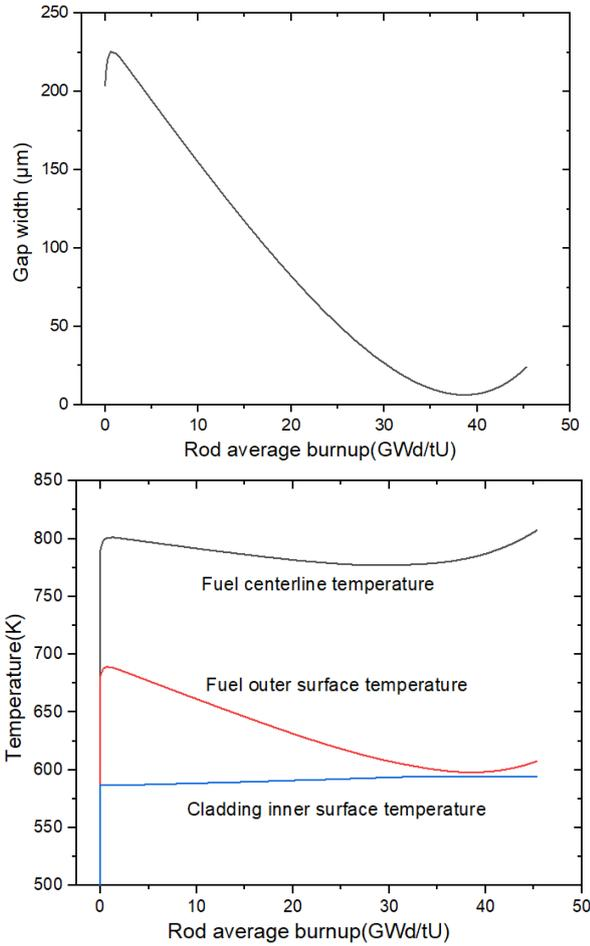
Fig. 3. (a) Gap size evolution and (b) fuel temperature profile at the middle axial region of fuel column
