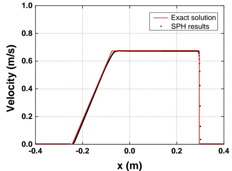
[ Velocity profiles (t=0.2 s, **ASPH O**) ]
