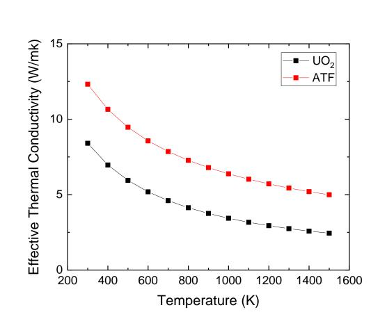
► The comparison of calculated effective thermal conductivity of 5 vol% containing micro-cell UO<sub>2</sub> and that of pure UO<sub>2</sub> calculated by the modified NFI model
