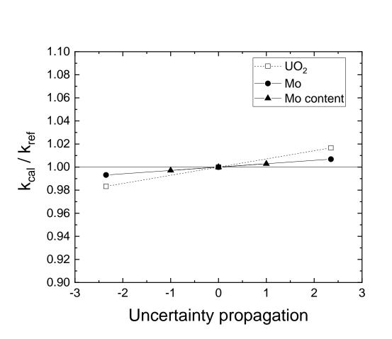
The combined uncertainty analysis was performed by using a random sampling method for parameters of the effective thermal conductivity of micro-cell UO<sub>2</sub> pellet.
