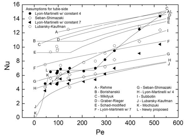
Fig. 2. Shell-side convective heat transfer characteristics in STELLA-1 sodium-to-sodium heat exchanger.
