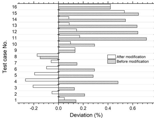
Fig. 5. Change in deviations of tube-side outlet temperature by use of proposed heat transfer correlation.
