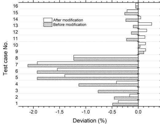
Fig. 4. Change in deviations of shell-side outlet temperature by use of proposed heat transfer correlation.
