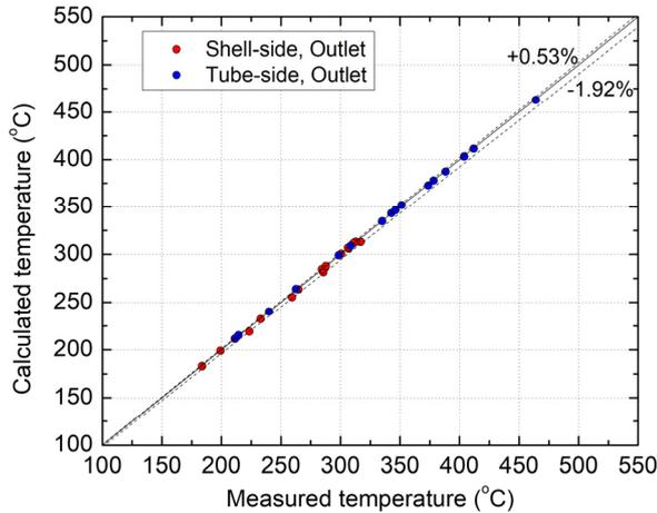
Fig. 3. Comparison of outlet sodium temperatures in STELLA-1 DHX experiment and SHXSA calculation.
