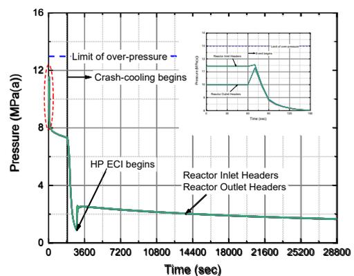
Fig. 2. Pressure of reactor headers.
