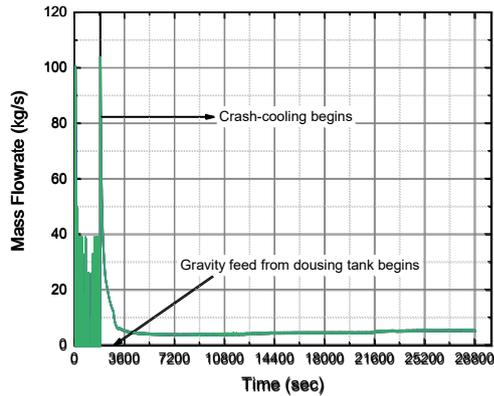
Fig. 3. Steam discharge flow through MSSVs.
