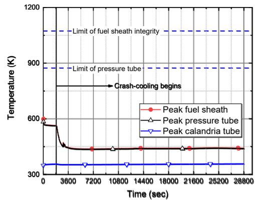
Fig. 5. Maximum temperature of fuel sheath and PT.
