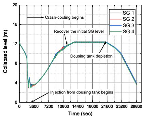
Fig. 4. Collapsed water level of SGs.
