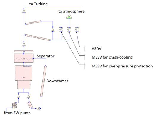
Fig. 1. SG model for simulating crash cooling.
