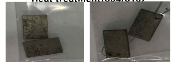
No Heat treatment(304/316) 도금완료
