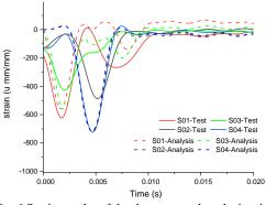
Fig. 6 Strain results of the drop test and analysis with the misaligned position
