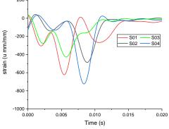
Fig. 2 Strain results of the drop test in the bottom drop (Cut-off frequency 300 Hz)
