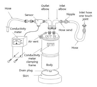
Fig. 2. An assembly diagram of the C-5P type ion exchanger
