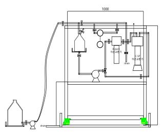
Fig. 1. Schematic diagram of ion exchange resin saturation loop developed in this work
