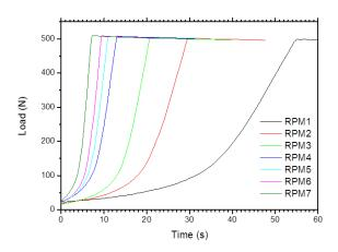
Fig. 1. Load obtained tensile test performed at room temperature with different RPM of motor.
