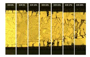
Fig. 2. Low magnification of inner- and outer-surface oxide layers for zircaloy-4 cladding oxidized at 1200C with different oxidation time.
