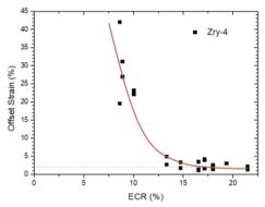
Fig. 4. Offset strain measured after ring compression test for cladding samples with different ECR.
