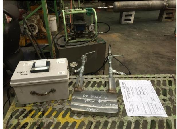
Fig. 5. Water pressure test of small mock-up (Part-C).
