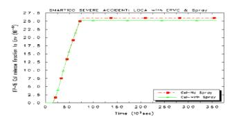
Fig. 2.3.1 CsI release fraction to environment
