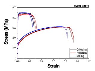
Fig. 4. Stress-strain curves of as-received material and 35% cold work material with different surface finishing method
