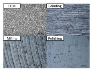
Fig. 3. Surface conditions of miniature tensile specimens with different surface processing method
