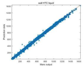
Figure 12 Wall heat transfer coefficient film regime with data augmentation
