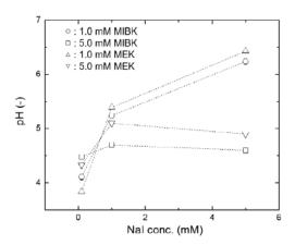
Fig. 3. pHs of NaI and methyl alkyl ketone (MIBK and MEK) mixed solutions after irradiation with 40 kGy gamma radiation [5]
