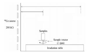
Fig. 1. Schematic diagram of gamma irradiation system [3,4]
