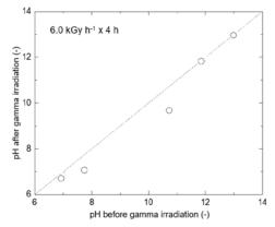
Fig. 2. pHs of NaOH solutions before and after gamma irradiation. The gamma doses were 24 kGy [5].
