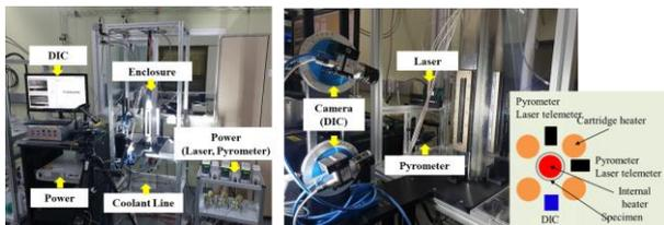
Fig. 3. Photo of NEST-1 and the configuration for performance test
