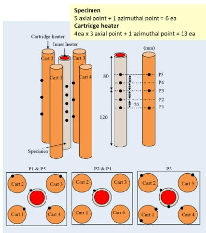
Fig. 6. T/C welding locations for temperature distribution test of NEST-2
