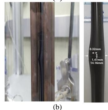
Fig. 5. Burst specimen during performance test
