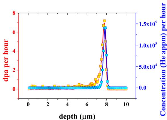
Fig. 2. SRIM/TRIM-predicted depth profiles of displacement per atom (dpa) per hour and induced He ion concentration in Fe per hour for the  $\text{He}^+$  beam acceleration test.
