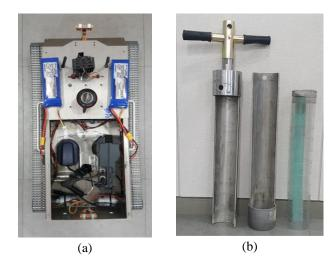
Fig. 1. The Measurement System for detecting concentrations of residual radioactivity
