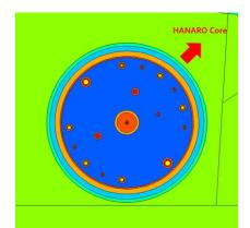
Fig. 2. Selected SPND arrangement (MCNP model)
