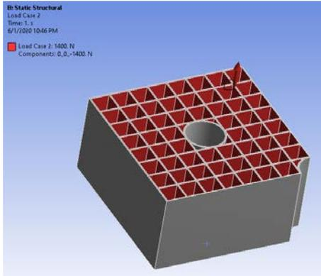
Figure 5 Force boundary condition with Hydraulic force
