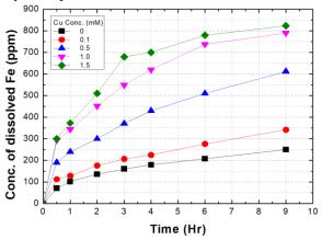
Fig 2. Dissolution behavior of magnetite according to the concentration of Cu ion.
