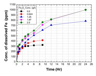
Fig 1. Dissolution behavior of magnetite according to initial input amount of magnetite.
