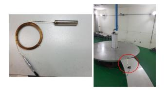
Fig. 3. Bias Gamma-ray Detector (left) and Gamma-ray irradiation test (right)
