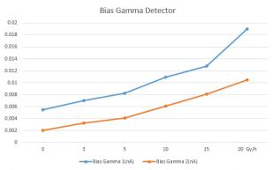
Fig. 5. Current measurement of bias gamma-ray detector.
