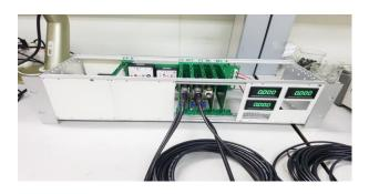
Fig. 4. Picoammeter for nA current measurement
