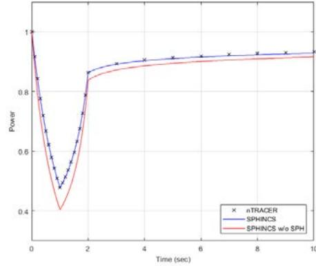
Fig.1. Necessity of generation of SPH factors with core power behavior for TD1-5 problem
