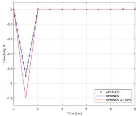
Fig. 2. Necessity of generation of SPH factors with reactivity change for TD1-5 problem
