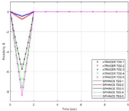
Fig. 8. Comparison of reactivity change for TD2 between SPHINCS and nTRACER
