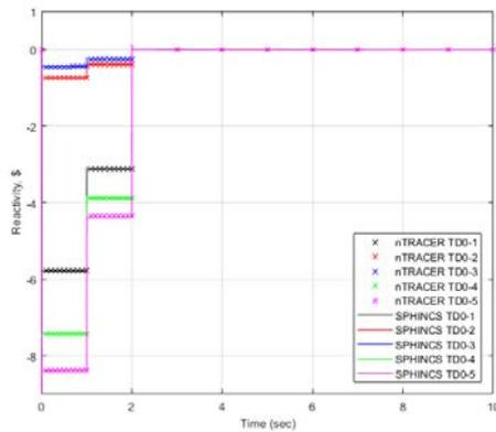
Fig. 4. Comparison of reactivity change for TD0 between SPHINCS and nTRACER
