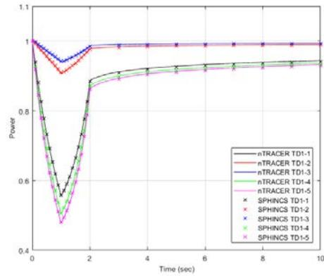
Fig. 5. Comparison of core power behavior for TD1 between SPHINCS and nTRACER
