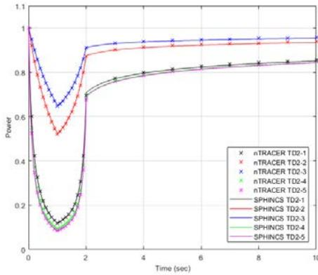
Fig. 7. Comparison of core power behavior for TD2 between SPHINCS and nTRACER
