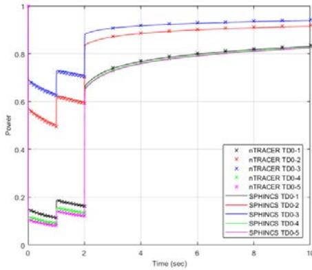
Fig. 3. Comparison of core power behavior for TD0 between SPHINCS and nTRACER
