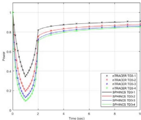
Fig. 9. Comparison of core power behavior for TD3 between SPHINCS and nTRACER
