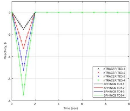
Fig. 10. Comparison of reactivity change for TD3 between SPHINCS and nTRACER
