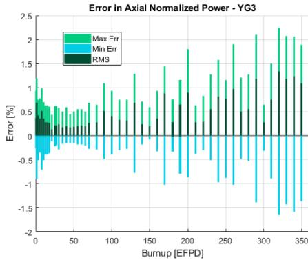
Fig. 8: RMS, MAX and MIN difference for each burnup steps of the YG3 reactor core.
