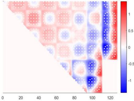
Fig. 2: axially integrated power difference between nTER standalone and nTER/ESCOT for Problem 5 (symmetry angle: 45).
