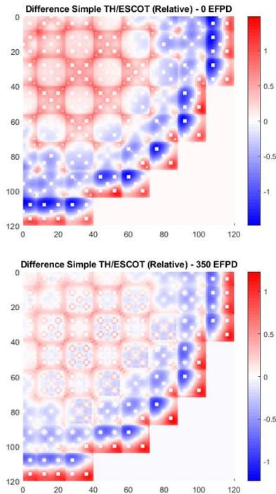
Fig. 7: axially integrated power difference for YG3 core at BoL (top) and EoC (bottom).
