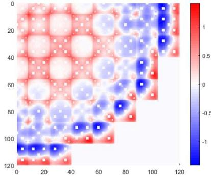
Fig. 4: axially integrated power difference between nTER standalone and nTER/ESCOT for YG3 core in case of activated CBC search mode (symmetry angle: 90).
