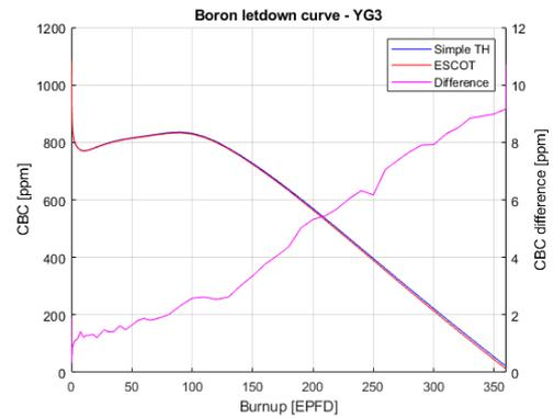
Fig. 5: boron letdown curve for YG3 core.
