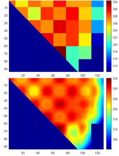
Fig. 3: outlet coolant temperature distribution for nTER standalone calculation (top) and nTER/ESCOT coupled platform (bottom).
