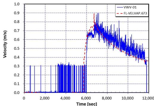
Fig. 5. Comparison of PAR inlet flow between test data and MELCOR prediction.
