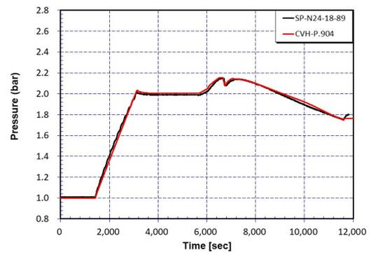
Fig. 3. Comparison of gas pressure inside the test vessel between test data and MELCOR prediction.
