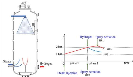
Fig. 1. Spray test in the SPARC test vessel (for the case of SSP test series).
