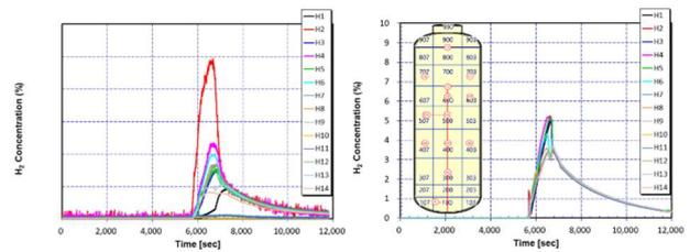
Fig. 6. Comparison of H<sub>2</sub> concentration inside the test vessel between test data and MELCOR prediction.
