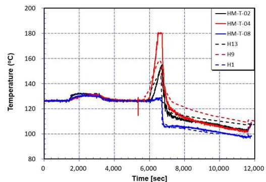
Fig. 4. Comparison of gas temperature inside the test vessel between test data and MELCOR prediction.
