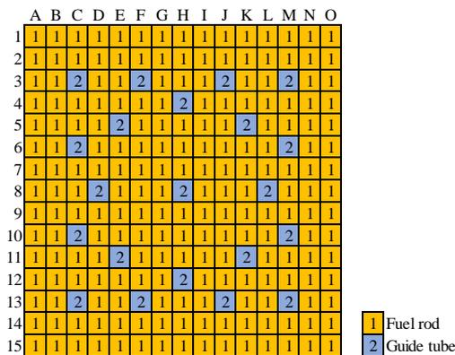
Figure 2 Layout of fuel assembly
