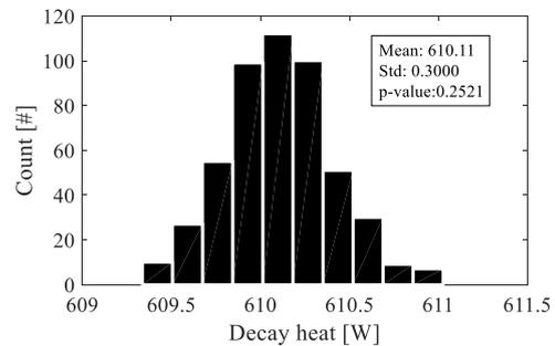
**Figure 5** Histogram of decay heat of B43 discharged from Turkey Point-3
