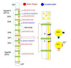
(a) Accelerometer and strain for fuel assembly vibration
