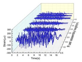
Fig. 2. Measured fuel assembly strain time history under simulated seismic accident under water, along the fuel height
