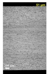
Fig. 1. Microstructure of Ti,Mo,C added 4th 136YTMC-2 alloy
