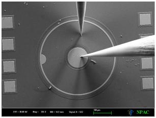
Fig. 3. SEM image of device measurement with e-beam irradiation using nano probe workstation
