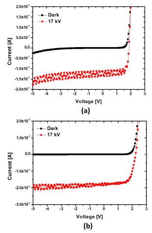
Fig. 4. I-V characteristics of Sample A(a) and B(b) w/ and w/o 17 kV e-beam irradiation
