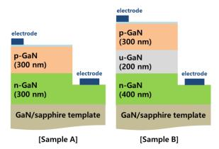
Fig. 1. Cross-sectional schematic of GaN betavoltaics fabricated on p-n (Sample A) and p-i-n junction (Sample B)
