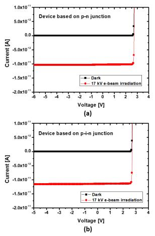
Fig. 5. Simulated I-V characteristics of devices based on p-n(a) and p-i-n junction(b)
