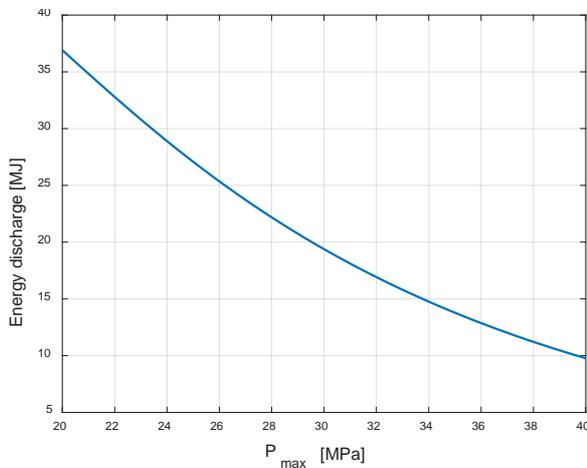
Fig. 11. Discharging energy change with respect to  $P_{max}$
