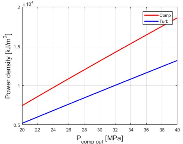
Fig. 6. Power density variation with respect to compressor outlet pressure
