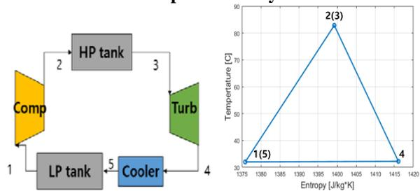
Fig. 2. Simple CCES layout and its T-S diagram
