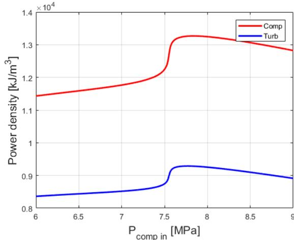
Fig. 4. Power density variation with respect to compressor inlet pressure
