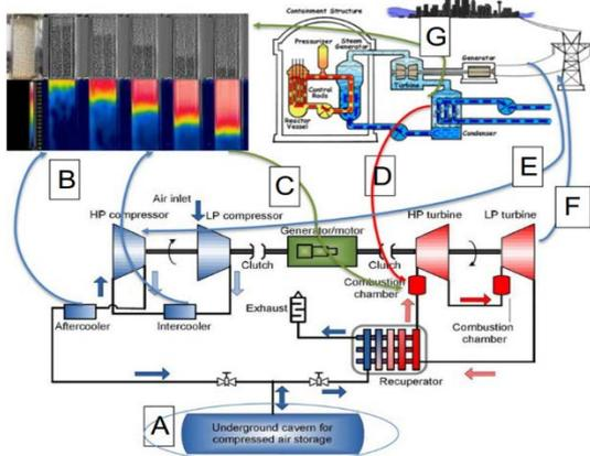
Fig. 1. Integration of energy storage system to nuclear power plant [1]
