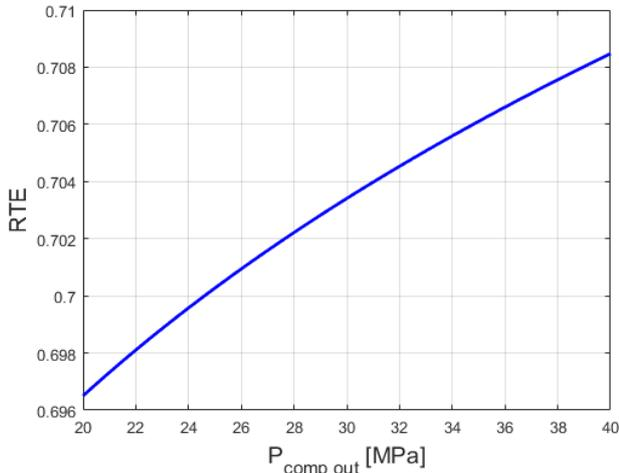
Fig. 5. Round-trip efficiency variation with respect to compressor outlet pressure
