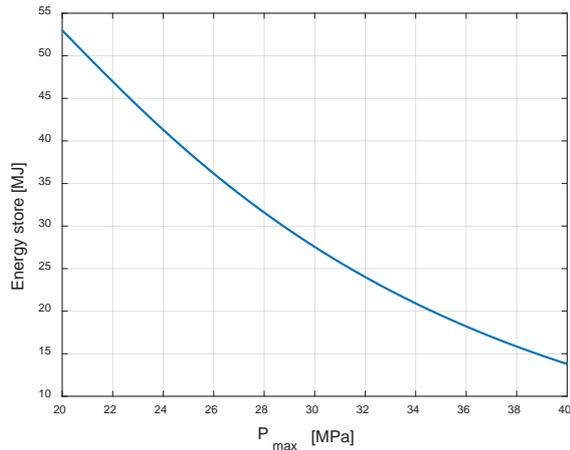
Fig. 10. Charging energy change with respect to  $P_{max}$
