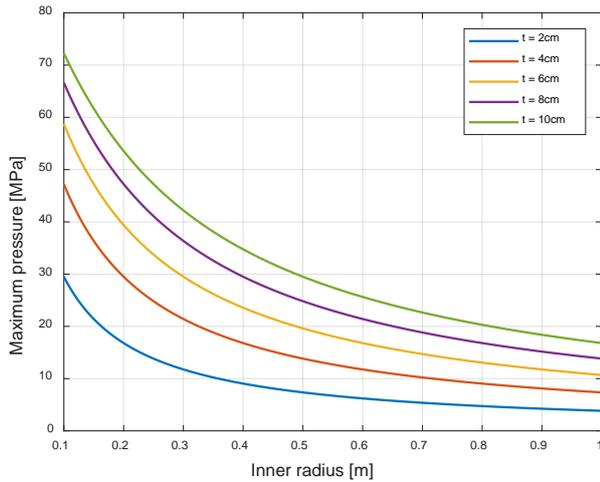
Fig. 7. Maximum pressure changes for pressure vessel
