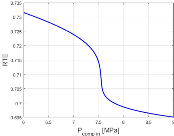
Fig. 3. Round-trip efficiency variation with respect to compressor inlet pressure
