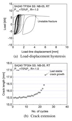
Fig. 3 Sample of data tested under load-controlled cyclic load
