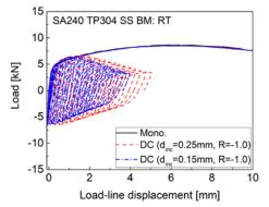
Fig. 2 Load-displacement curves of monotonic and displacement-controlled cyclic loads
