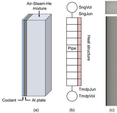
Fig. 3. Computational domain, nodalization of MARS-KS and computational meshes of CUPID for CONAN test simulation
