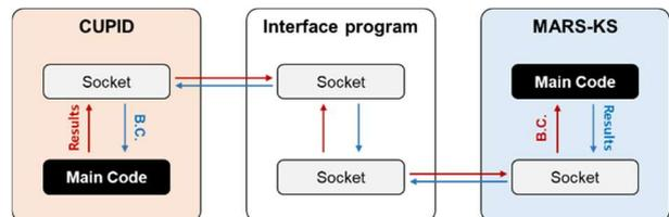
Fig. 1. MARS-CUPID code coupling with socket communication scheme
