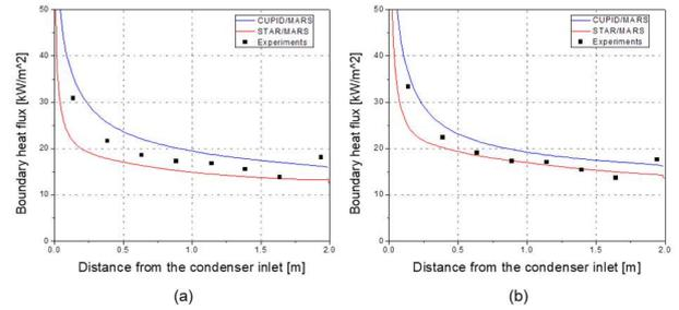
Fig. 4. Local condensation heat flux: forced convective condensation
