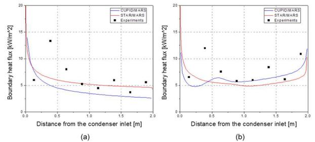
Fig. 5. Local condensation heat flux: natural convective condensation
