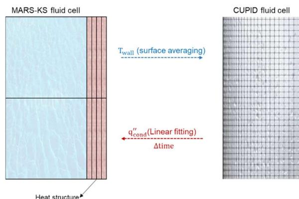
Fig. 2. MARS-CUPID heat structure coupling diagram
