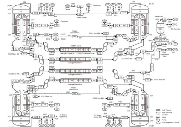
Fig. 2. Node system of general CANDU type reactor using M-CAISER
