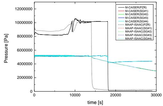
Fig. 3. Pressure of pressurizer and steam generator
