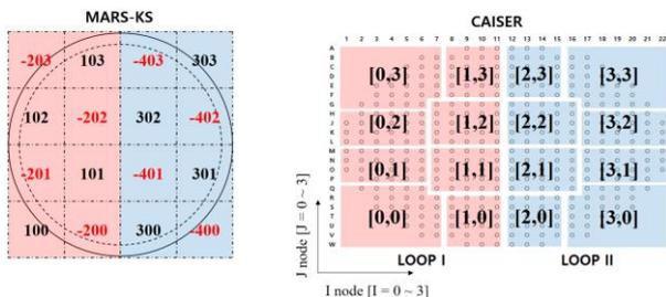
Fig. 1. Node mapping of reactor core at M-CAISER
