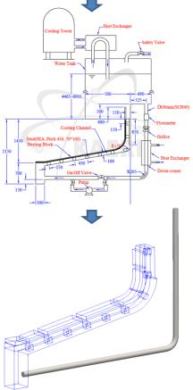
Fig. 3. CE-PECS test facility and geometrical modeling for a validation of the analytical method
