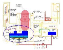
Fig. 1. Schematics of Core-Catcher for EU\_APR1400 [2].
