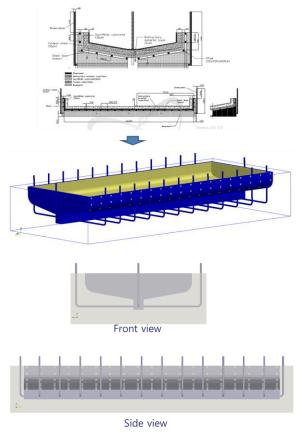
Fig. 2. Visualization of PECS using a 3D CAD data.
