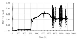
Fig. 4. Temporal flow rate of water flowing through down-comer of CE-PECS.
