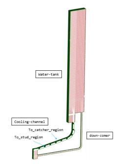
Fig. 4. Mesh system of CE-PECS test facility used for a preliminary analysis.
