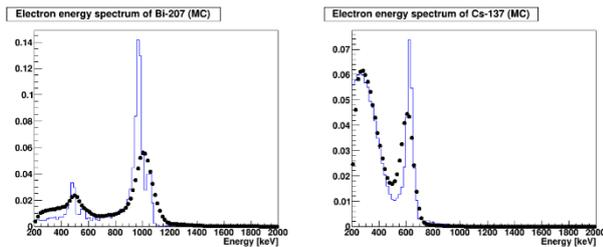
Fig. 8. Comparison of measurements (black dots) and simulation calculations (blue line) before applying energy resolution.
