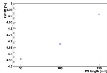
Fig. 7. Energy resolution according to plastic scintillator thickness.
