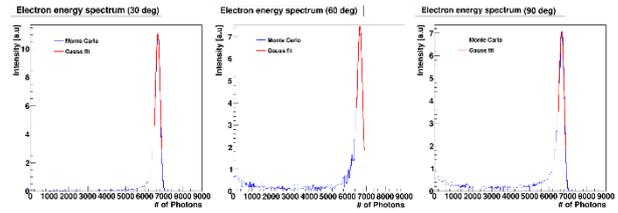
Fig. 4. The electron energy spectra according to the solid angle (blue line) and Gaussian fitting of the peaks (red line). The x-axis is the number of photons generated in the plastic scintillator corresponding to the energy. The y-axis is the intensity when the total area of the spectrum is 100.
