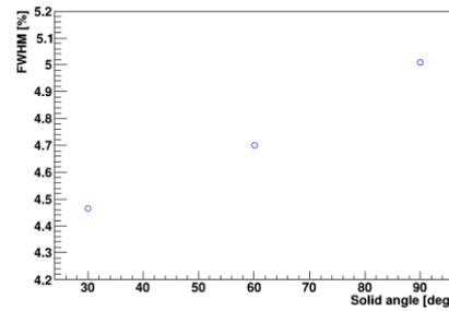
Fig. 5. The energy resolution according to solid angle.
