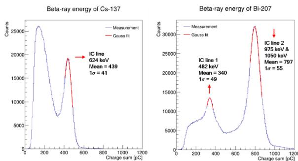
Fig. 3. The beta-ray energy spectra of  $^{137}\text{Cs}$  (left) and  $^{207}\text{Bi}$  (right) sources. The x-axis is the area (charge quantity) of the signal.
