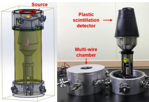
Fig. 1. The beta-spectrometer.
