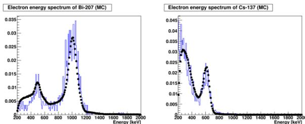
Fig. 9. Comparison of measurements (black dots) and simulation calculations (blue line) after applying energy resolution.
